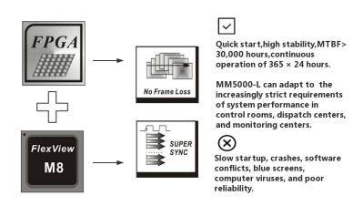
MM5000-L adopted the 4th generation hardware processing architecture and Flexview M8 algorithm supports pixel by pixel output, receiving multiple 4K/8K signals sources, and real-time processing without frame loss. With the help of high speed paralleled processing, super sync and full frame technologies, the processor guarantees all outputs in super sync and no image tearing.
